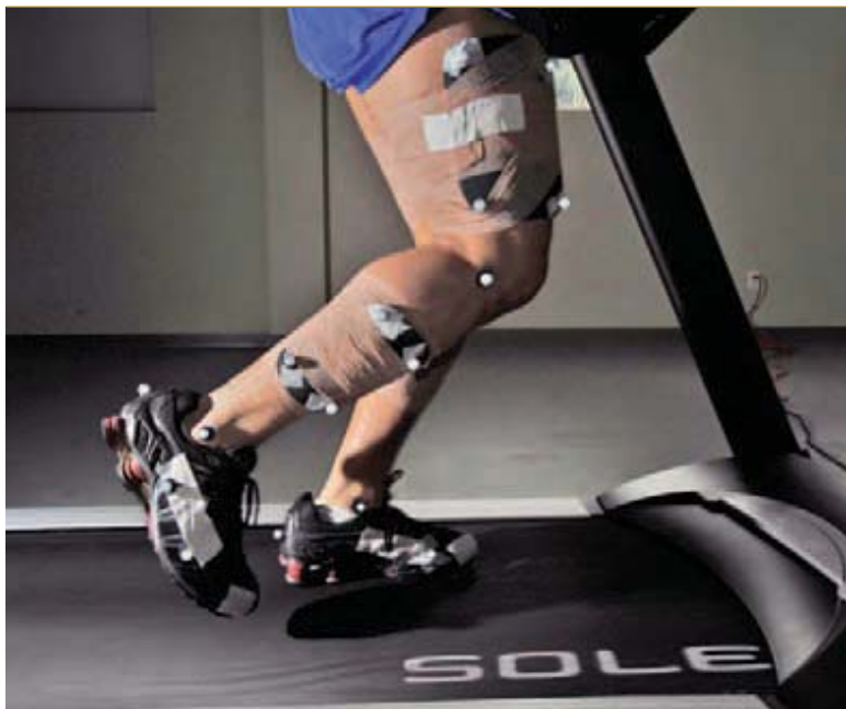
A study volunteer runs on a treadmill in the Gait and Motion Analysis Lab at the Center for Restorative and Regenerative Medicine, his legs taped with reflective markers that are tracked by motion-capture cameras. Meanwhile, researchers check the results from software that creates a 3D representation of the volunteer's leg movements.
